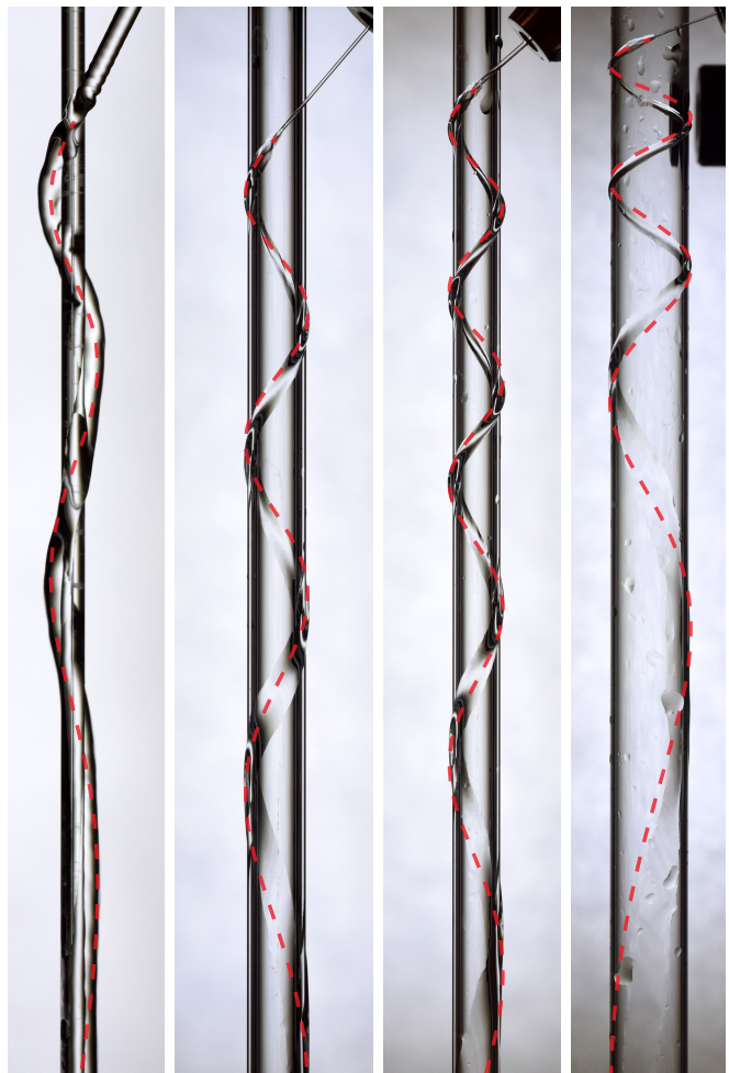
FIG. 3. Comparison between experiments and theory for a range of experimental parameters. From left to right: D_t = 1, 5, 5, 10 mm, D_j = 1, 0.3, 0.5, 0.3 mm; \psi = 26.3, 40.3, 47.8, 68.6 deg; U_0 = 1.0, 4.9, 3.0, 5.4 m/s; C = 15, 11.5, 7, 9.5 .
