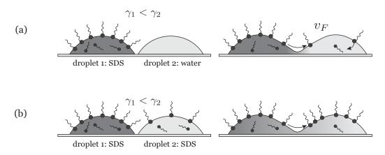
FIG. 8. Mechanism of lifetime difference between cases (a) and (b) explained. Panels (a) and (b) show the difference in surfactant coverage. Panel (b) shows the accumulation of surfactants at the surface of droplet 2 in a schematic way. In all images, the size of the surfactant molecules is exaggerated as well as the number of surfactants at the interface as compared to the bulk.
