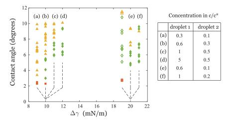
FIG. 5. Phase diagram of two coalescing droplets of different SDS concentrations; the same legend as in Fig. 4 applies for the regimes. Several concentration couples are used to obtain series at  $\Delta \gamma = 10 \text{ mN/m}$  and 20 mN/m. From left to right, we move to higher concentrations. The table specifies the concentrations, in terms of the critical micelle concentration  $c^*$ . The open symbols at 20 mN/m represent the water-SDS case from Fig. 4, included for comparison.
