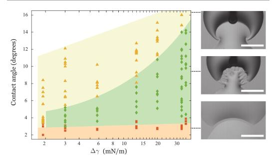
FIG. 4. Phase diagram of the coalescence behavior of a water drop and an SDS drop. Both the surface tension difference  $\Delta \gamma$  and contact angle are varied. Red squares, vapor- and/or precursor-mediated interaction; green diamonds, fingering instability; yellow triangles, stable delayed coalescence. The color regions are intended as a guide to the eye. The insets show enlargements of the top view of the contact region between the two drops (scale bars: 3 mm).
