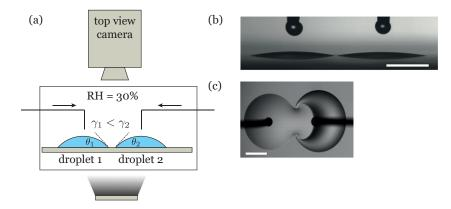
FIG. 1. (a) Cross-sectional sketch of the experimental setup, defining the parameters  $\theta_i$  and  $\gamma_i$ . Panels (b) and (c) show typical images obtained from side- and top-view cameras, respectively. In both images, the scale bar represents 3 mm. The left droplet is pure water; the right droplet contains SDS. Note that in the top view the needle visible in the image is no longer in contact with the droplets.
