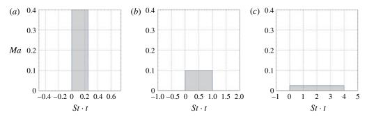
FIGURE 7. (Colour online) Three ablation pressure pulses of different duration but constant impulse (MaSt = 0.1). (a) A short pulse with a duration St = 0.25 and amplitude Ma = 0.4, (b) an intermediate pulse duration St = 1 and Ma = 0.1 and (c) a long pulse duration St = 4 and Ma = 0.025.
