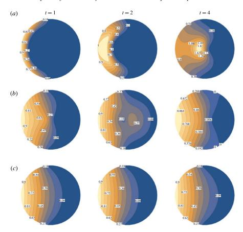
FIGURE 9. (Colour online) The pressure impulse field  $J_1$  inside the droplet for the three different pulse durations illustrated in figure 7: (a) St = 0.25, (b) St = 1 and (c) St = 4. The results are depicted for different times: at the end of the pulse (t = 1), at two times the pulse duration (t = 2) and at four times the pulse duration (t = 4). Note that the colour bar scale is not fixed and that all fields are scaled with  $p_e \tau_e$ .
