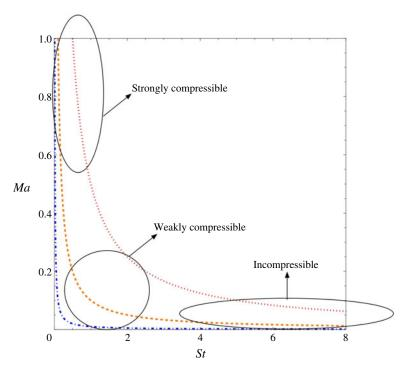
FIGURE 3. (Colour online) A phase diagram showing lines of constant impulse transfer to the droplet. The blue dotted-dashed line is the isoline St Ma = 0.01, the orange dashed line is the isoline St Ma = 0.5. The plot shows three distinct regimes can be observed at constant impulse: a strongly compressible regime, a weakly compressible regime and an incompressible regime. The weakly compressible regime is the focus of the present work.
