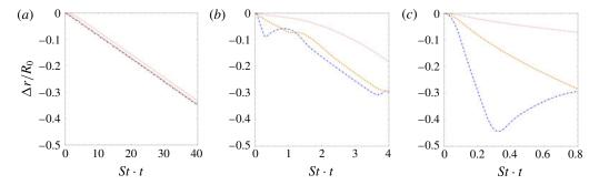
FIGURE 12. (Colour online) The advective displacement of the droplet interface  $\Delta r/R$  at the axis of impact  $(r=1, \theta=0)$  for the three different pulse durations: St=0.25 (blue dot dashed), St=1 (orange dashed) and St=4 (red dotted). (a) MaSt=0.01, (b) MaSt=0.1 (c) MaSt=0.5.
