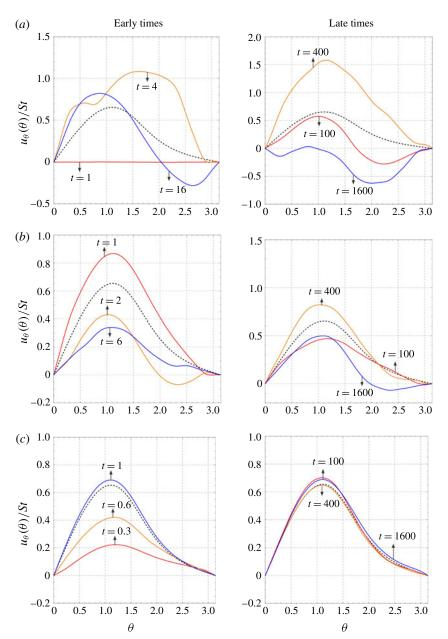
FIGURE 10. (Colour online) The  $\theta$  component of the velocity field inside the droplet at r = 0.5. The left column represents early times  $(t \sim 1)$  while the right column represents late times  $(t \gg 1)$ . (a) A short pulse duration St = 0.25, (b) an intermediate pulse duration St = 1 and (c) a long pulse duration St = 4. The black dashed line denotes the incompressible velocity field by Gelderblom et al. (2016).
