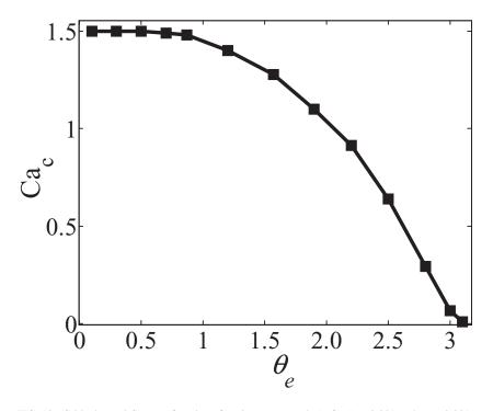
FIG. 12. Critical speed Ca<sub>c</sub> as a function of static contact angle  $\theta_e$  for R=0.001 and  $\lambda_s=0.001$ .
