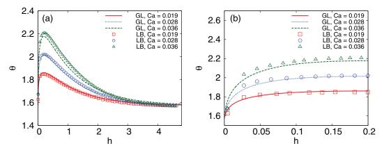
FIG. 5. Local meniscus angle  $\theta$  vs h for R = 1. Identical parameters as in Fig. 4.
