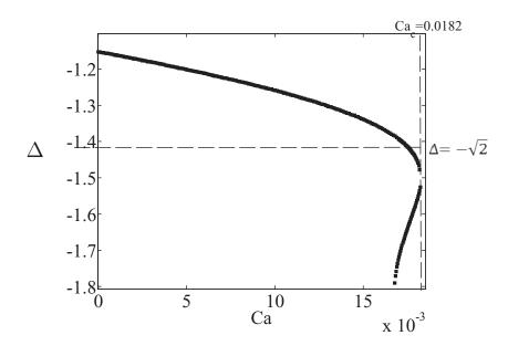
FIG. 6. Meniscus fall  $\Delta$  versus Ca ( $\theta_e = 2.8$  rad, R = 0.01,  $\lambda_s = 10^{-5}$ ). The horizontal dashed line indicates the minimum value of  $\Delta$  for a static meniscus ( $= -\sqrt{2}$ , with  $\theta_e = \pi$ ).
