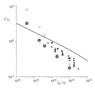
FIG. 13. Figure extracted from Ref. 8. Dimensionless entrainment (critical) speed, denoted as  $Ca_e$  versus the viscosity ratio  $\eta_g/\eta_\ell$  for silicon-oil/air ( $\bullet$ ,  $\diamond$ , data from Ref. 8), silicon-oil/air ( $\blacksquare$  data from Ref. 6), and various liquids/air ( $\blacktriangle$  data from Ref. 11). Curve: Numerical results from our generalized lubrication model (slip length  $\lambda_s = 10^{-5}$ ,  $\theta_e = 50^\circ$ ).
