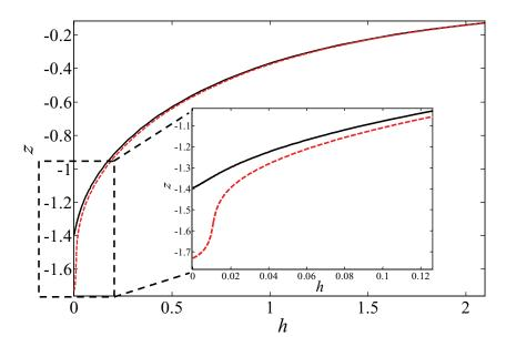
FIG. 7. Meniscus profiles for the upper branch (black solid curve) and the lower branch (red dashed curve) solutions for Ca = 0.017 ( $\theta_e = 2.8$  rad., R = 0.01,  $\lambda_s = 10^{-5}$ ). Here we define  $z = \Delta - x$ . So the bath level is at z = 0.
