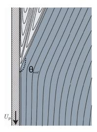
FIG. 2. Streamlines of the flow in a wedge of angle  $\theta_{wed}$ , which in this case is close to  $\pi$ . This flow solution has been derived analytically by Huh and Scriven, <sup>32</sup> and is used here to derive a generalized lubrication model.
