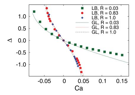
FIG. 3. Meniscus deformation  $\Delta$  as a function of Ca for  $\theta_e = \pi/2$ . Ca is negative/positive when the plate is moving upward/downward. Symbols: Results of Lattice Boltzmann (LB) simulation. Lattice separation = 0.01. Curves: Results of the lubrication-type (GL) model with a slip length  $\lambda_s = 0.002$ . All lengths are scaled by the capillary length  $\ell_{\gamma}$ .
