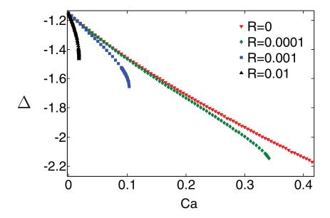
FIG. 8. Meniscus fall  $\Delta$  versus Ca for different viscosity ratios ( $\theta_e = 2.8 \text{ rad}$ ,  $\lambda_s = 10^{-5}$ ). For the case the gas phase has no viscosity, R = 0, steady-state menisci can be maintained to arbitrarily large velocity (within our numerical resolution).
