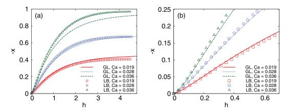
FIG. 4. Dynamical meniscus profiles -x vs h for R=1 ( $\theta_e=\pi/2$  and  $\lambda_s=0.002$  for the GL model, lattice separation = 0.01 for the LB simulation). All lengths have been scaled by the capillary length. The contact line is at x=0 so that the bath is at different x for different Ca. (a) Curves: Results of GL model. Symbols: Results of LB simulation. (b) Zoom in on the contact line region.
