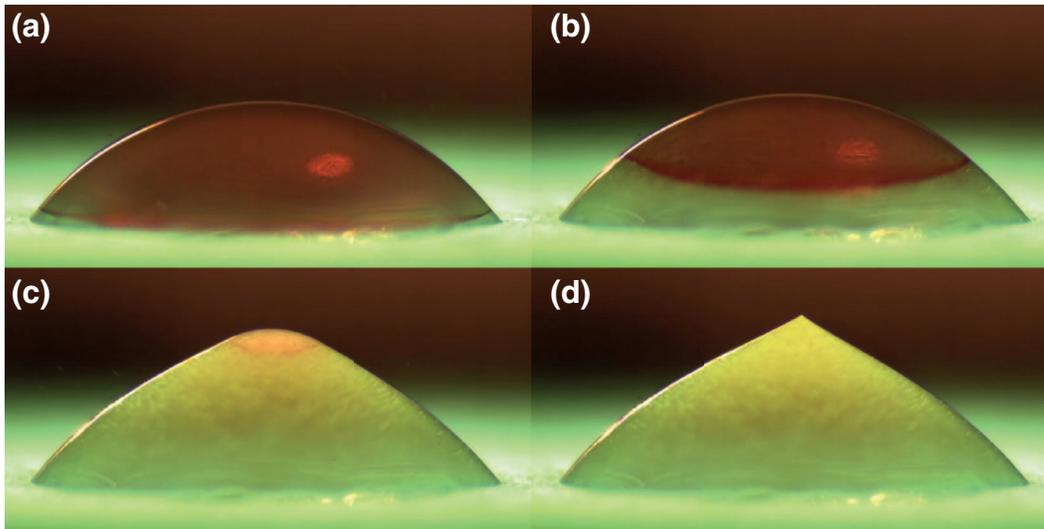
FIG. 1. Four snapshots of the freezing process of a drop of water on a cold plate ( $T = -20^{\circ}\text{C}$ ). The freezing front travels from bottom to top in about 18 s. The time between the snapshots is 4.6 s (a) and (b), 11.42 s (b) and (c), and 1.28 s (c) and (d). The droplet radius at the base is approximately 2 mm. During the final stage of the freezing process, the ice drop develops a singular shape with a pointy tip (enhanced online) [URL: <http://dx.doi.org/10.1063/1.4747185.1>].
