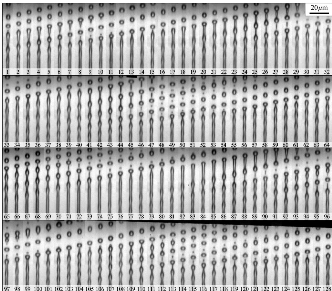
FIG. 9. A sequence of 128 image frames recorded at 13.76 Mfps showing the breakup of a  $1.25 \mu\text{m}$  radius liquid jet into microdroplets. The liquid used was a 0.9% saline solution with density  $\rho=1003 \text{ kg/m}^3$ , surface tension  $\gamma=72 \text{ mN/m}$ , and viscosity  $\eta=1 \text{ mPa s}$ . The frame number is indicated in the bottom of each frame. The interframe time is 73 ns.
