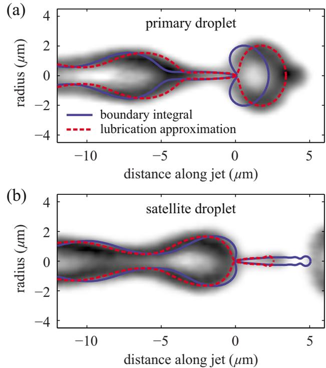
FIG. 12. (Color online) Comparison between the boundary-integral simulation and the one-dimensional lubrication approximation for the breakup of a  $1.25 \mu\text{m}$  jet. The jet velocity is  $35 \text{ m/s}$ . A 0.9% normal saline solution was used with density  $\rho_\ell = 1003 \text{ kg/m}^3$ , viscosity  $\eta = 1 \text{ mPa s}$ , and surface tension  $\gamma = 72 \text{ mN/m}$ .
