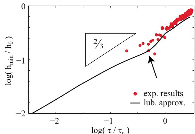
FIG. 6. (Color online) The logarithm of the normalized minimum radius of the neck  $h_{\text{min}}/h_0$  as a function of the logarithm of the time remaining until droplet pinch-off  $\tau = t_c - t$ , normalized by the capillary time  $\tau_c$ , scales with a characteristic  $2/3$  scaling exponent.
